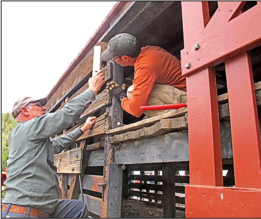
Volunteers work on restoration of double-deck stock car No. 5543 that hauled sheep, cattle and hogs, built in 1904 by the American Car and Foundry Company. The replacement replica stock car door partially funded by the Rocky Mountain Railroad Historic Foundation grant is on the right. – Photo © 2021 Joe Becker.
